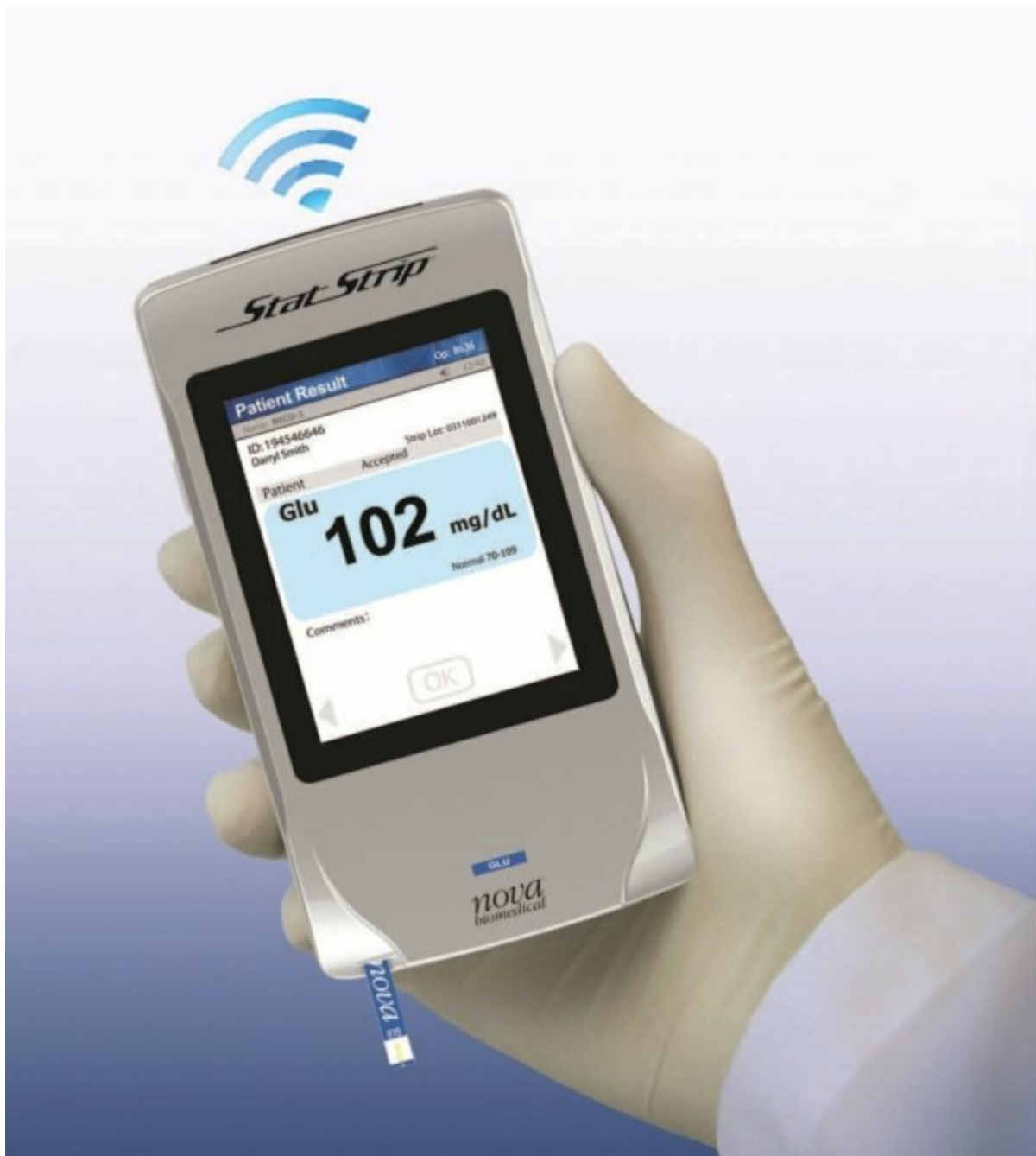
FIGURE 11-24. Nova BioMedical StatStrip® with wireless connectivity. (Courtesy of Nova BioMedical, Waltham, Massachusetts, USA.)
