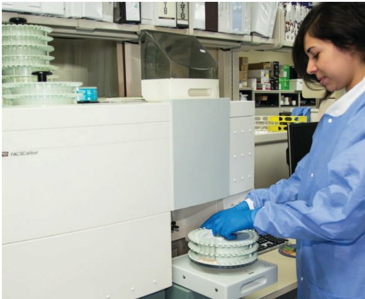
FIGURE 1-15. Medical Laboratory Scientist loads BD FACSCalibur™ modular flow cytometry analyzer with tissue samples for HLA testing.
